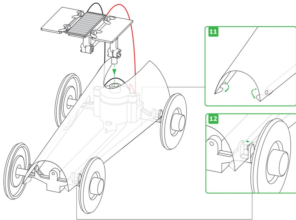
11. There is also a transparent plastic body sheet provided in this kit that you can use to make a body shell. Fold the plastic sheet along the edges as diagram.
