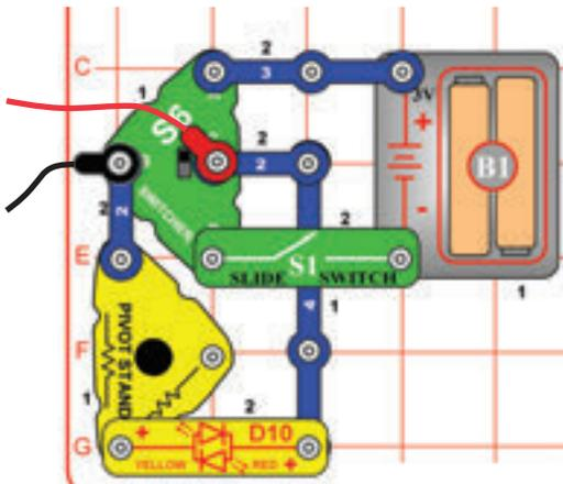
Modify the preceding circuit to include the red/yellow bicolour LED (D10), which lights yellow when the crawler is going forward, or red with it goes backward.
