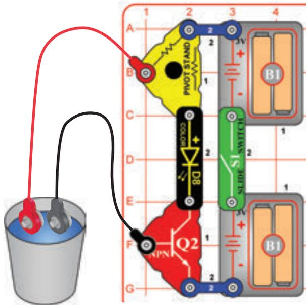
Build the circuit and turn on the switch (S1). Touch the metal in the jumper wire snaps with your fingers; the color LED (D8) should light. If the LED is dim or off, hold the metal more tightly or wet your fingers.
