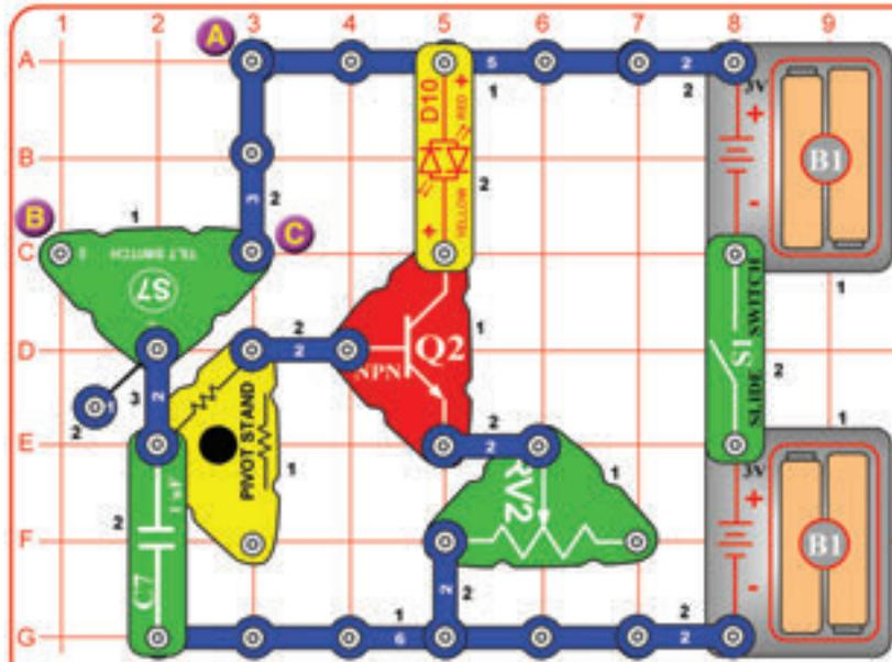
When tilt is detected, the 1µF capacitor (C7) is charged through the tilt switch (S7). When tilt is removed, the capacitor discharges through the resistors in the pivot stand and RV2, and through the NPN transistor (Q2). The light stays on as the capacitor discharges. RV2 also limits the current through the LED (D10), and so affects the LED brightness.
