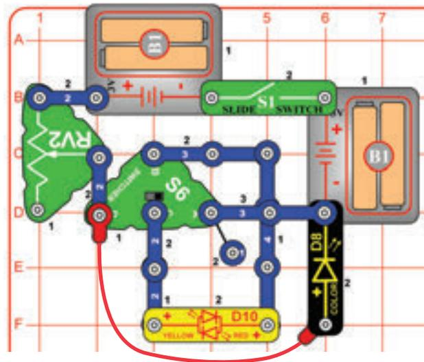
Build the circuit and turn on the slide switch (S1). Use the switcher (S6) to set the color of the red/yellow bicolor LED (D10) and use the adjustable resistor (RV2) to set the brightness of the LEDs.
