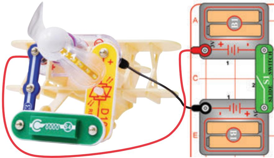
Note: This circuit has the red/yellow bicolor LED (D10) connected directly across the batteries without another component to limit the current. Normally this might damage the LED, however Boffin LEDs have internal protection resistors to protect them from incorrect wiring, and will not be damaged.
