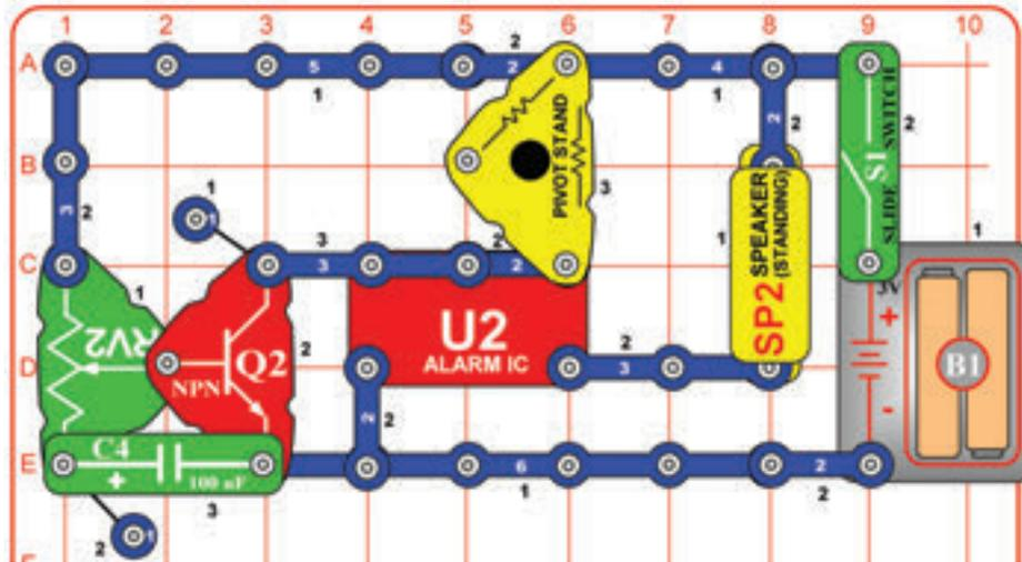
Set the adjustable resistor (RV2) to the bottom position. Turn on the slide switch (S1). A machine gun sounds for a second, then stops. Turn off the slide switch, wait a few seconds, then turn it back on to hear the machine gun sound again. Try this several times.
