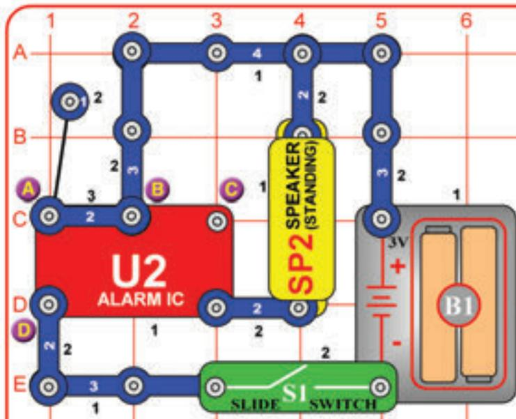
Build the circuit and turn on the slide switch (S1). You hear a siren.
