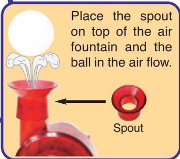
Build the circuit as shown, place the spout on the air fountain (AF), turn on the slide switch (S1), then place the ball directly in the blowing air above the air fountain. The blowing air should balance the ball, so it floats in the air and “dances”. Occasionally the ball may become unstable and fall out; just place it back into the air flow.
