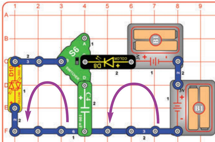
Set the switcher (S6) to the top position; the color LED (D8) flashes. Now set S6 to the bottom position; the red/yellow bicolor LED (D10) flashes red. Alternate setting S6 to top and then bottom. The middle S6 position is "off".
