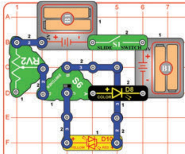
The color LED (D8) contains separate red, green, and blue lights, with a micro-circuit controlling them. The controlling circuit briefly turns the LED off between colors, which also shuts off the red/yellow LED because both are connected in series.
