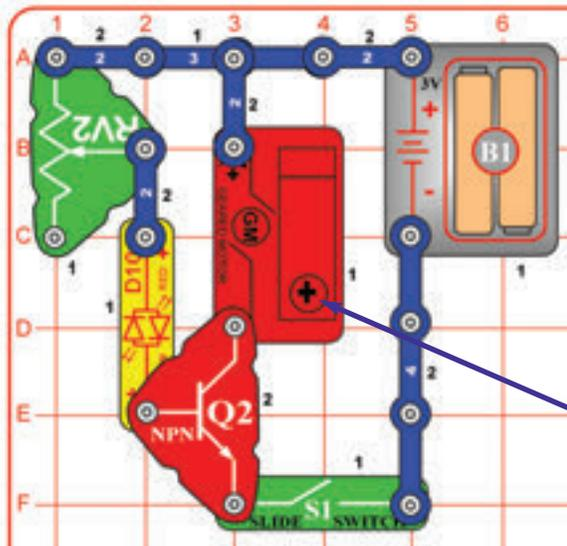
Insert some of the cardboard figures into the 3 slots on the edge of the merry-go-round base. Build this circuit and mount the merry-go-round base onto the shaft on the geared motor (GM).
