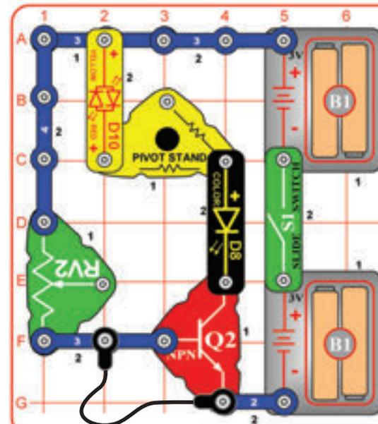
Build the circuit shown and turn on the slide switch (S1). Nothing happens. Break the black jumper wire connection and lights flash. You could replace the black jumper wire with a longer wire and run it across a doorway to signal an alarm when someone enters.
