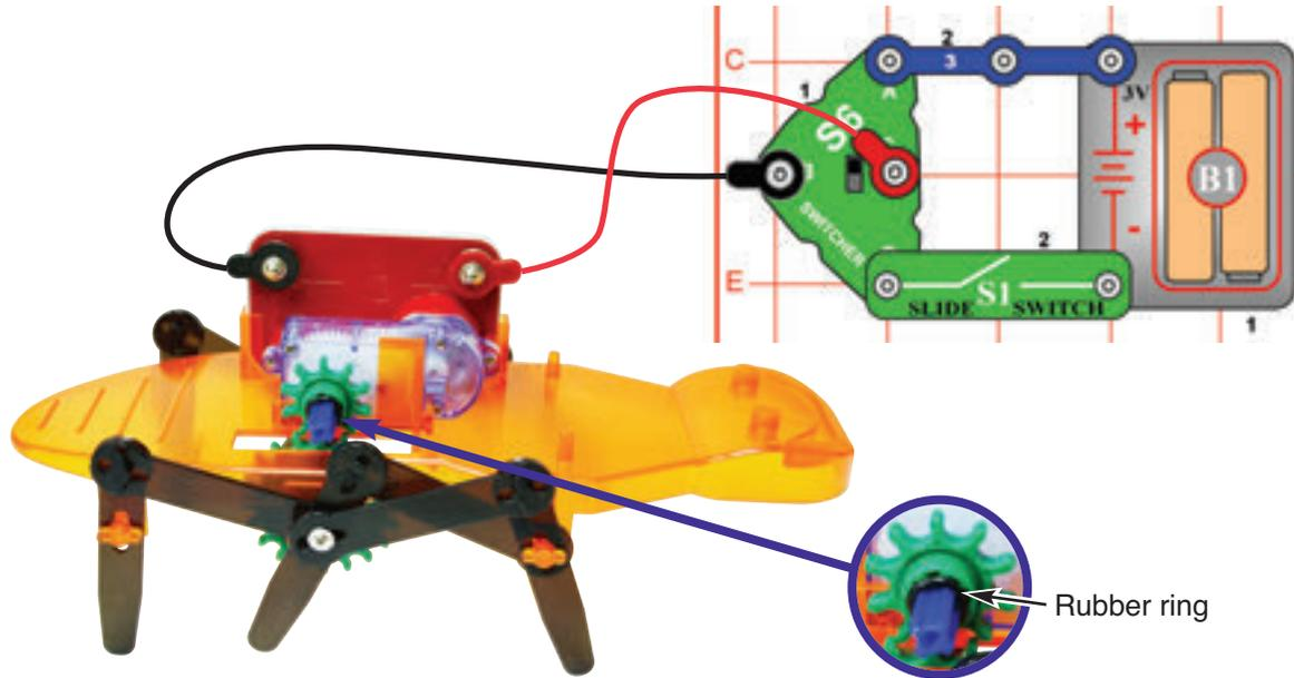
Assemble the crawler using the assembly instructions on pages 6 and 7, and build the circuit shown here. Mount the smallest gear (1.0") on the geared motor (GM) with a rubber ring to keep it from sliding out of position, place it on the crawler frame, and connect it to the circuit using the red & black jumper wires.
