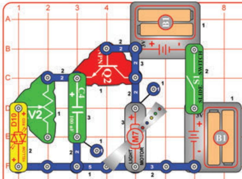
Turn on the slide switch (S1). The red/yellow bicolor LED (D10) and light motor (M7) are on. The adjustable resistor (RV2) sets the brightness for D10.
