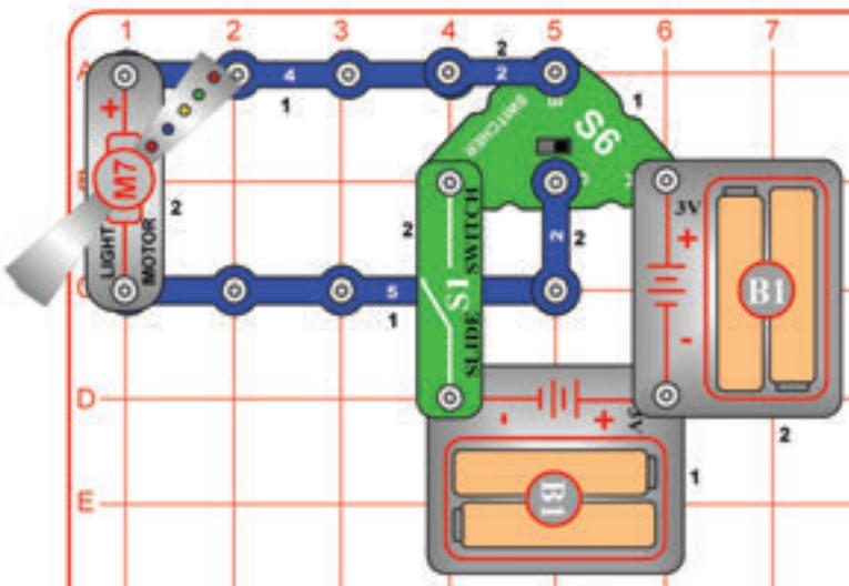
Build the circuit, turn on the slide switch (S1), and set the switcher (S6) to the left or right to control the light motor (M7).
