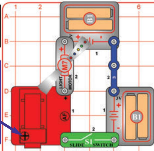
Motors need lots of electric current when they start up, then much less when their shafts are spinning at high speed (it is harder to get the shaft spinning than to keep it spinning). Compare this to riding a bicycle: you have to pedal harder to get going, then it's easy to keep going at a constant speed.
