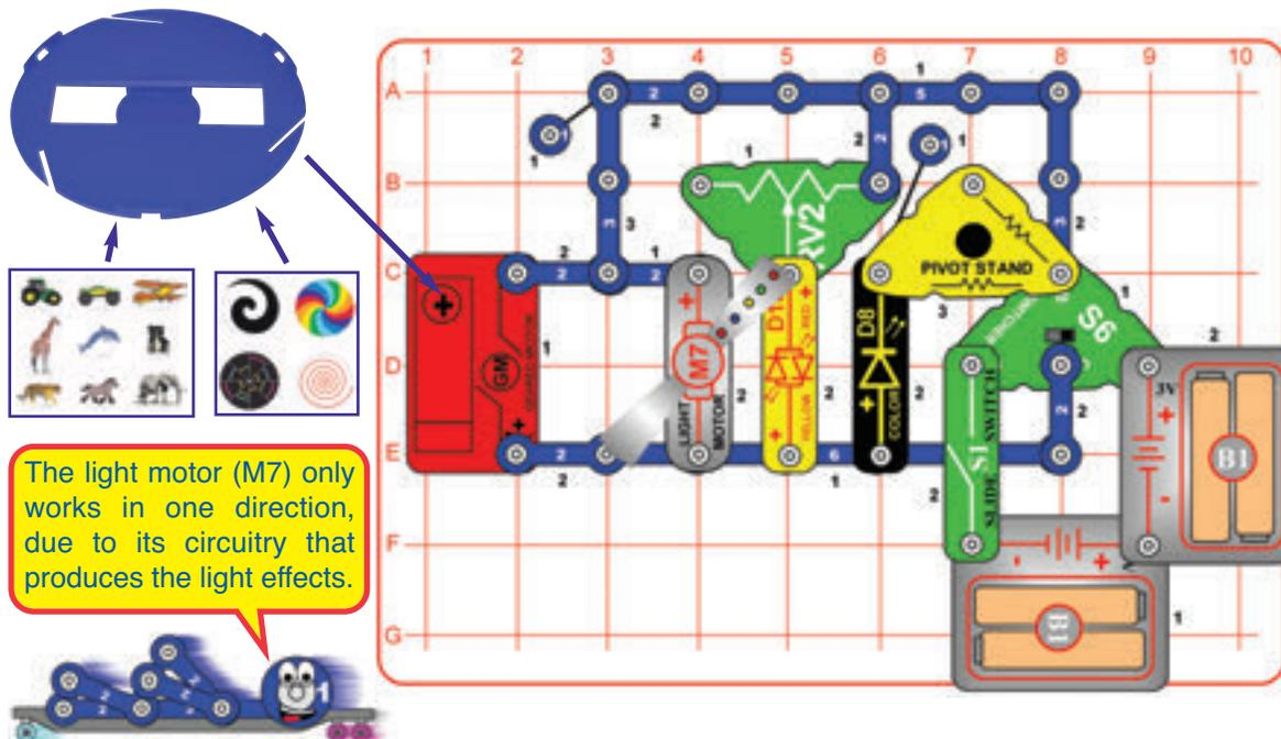
The light motor (M7) only works in one direction, due to its circuitry that produces the light effects.
