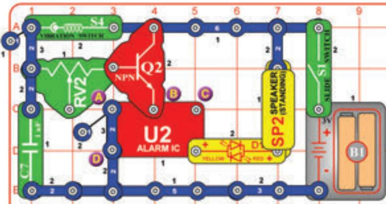
Build the circuit as shown. Tap on the vibration switch (S4) or bang on the table to activate an alarm and make the red/yellow LED (D10) light.
