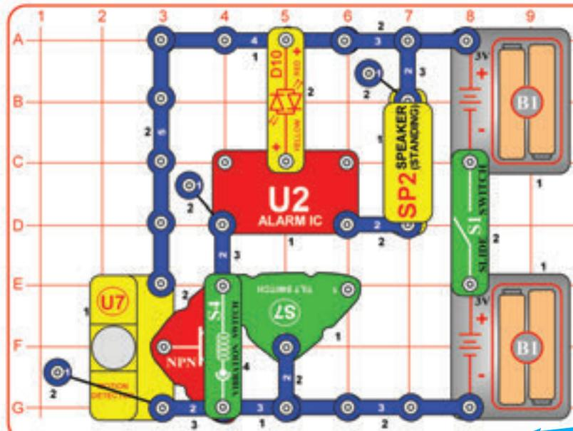
Assemble the circuit and place the base grid into the blue stand (with the NPN transistor (Q2) closest to the stand) and carefully stand it up. Position it near the edge of a table, facing across a room.
