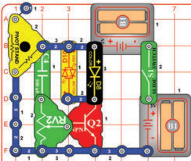
Set the adjustable resistor (RV2) to the top setting. Turn on the slide switch (S1). The LEDs (D8 & D10) light for a few moments. Now turn off the slide switch, wait a little while, and then turn it back on. The LEDs light briefly again. Try this several times.
