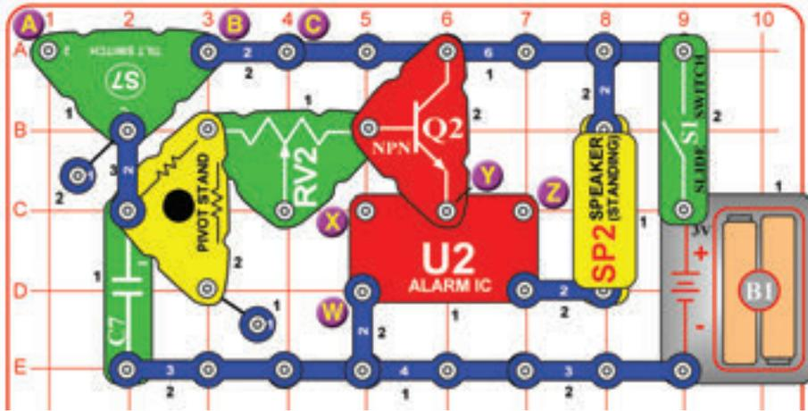
When tilt is detected, the 1µF capacitor (C7) is charged through the tilt switch (S7). When tilt is removed, the capacitor discharges through the resistors in the pivot stand and RV2, and through the NPN transistor (Q2). The alarm stays on as the capacitor discharges.
