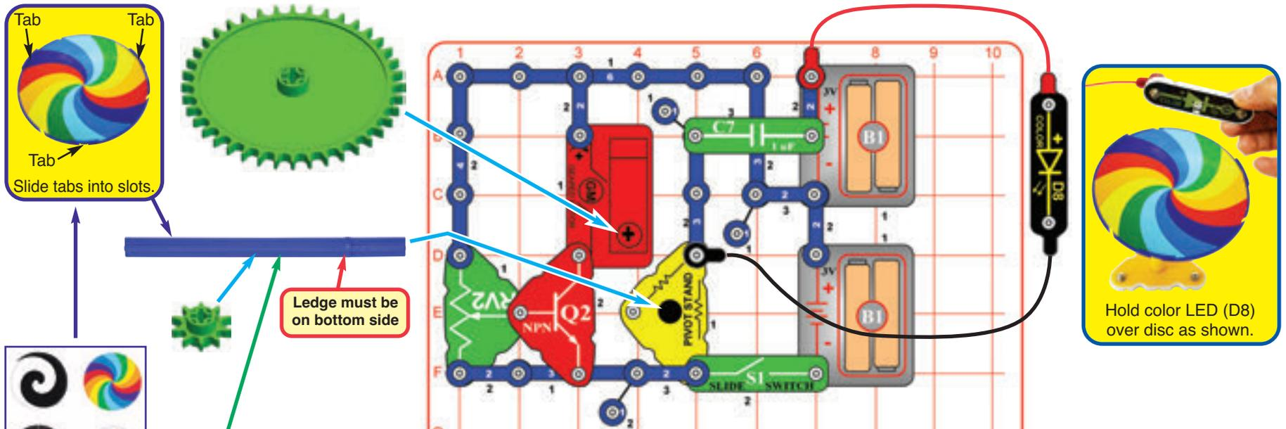
Build the circuit shown. Mount the 3.3" gear on the geared motor (GM), mount the 1.0" gear on the "+" shaped bar, place the "+" bar into the pivot stand, and then align the position of the 1.0" gear on the "+" shaft so the teeth of both gears mesh. Install one of the colored discs into the merry-go-round base. Mount the merry-go-round base onto the top of the "+" shaped bar. Connect the color LED (D8) using the red & black jumper wires.
