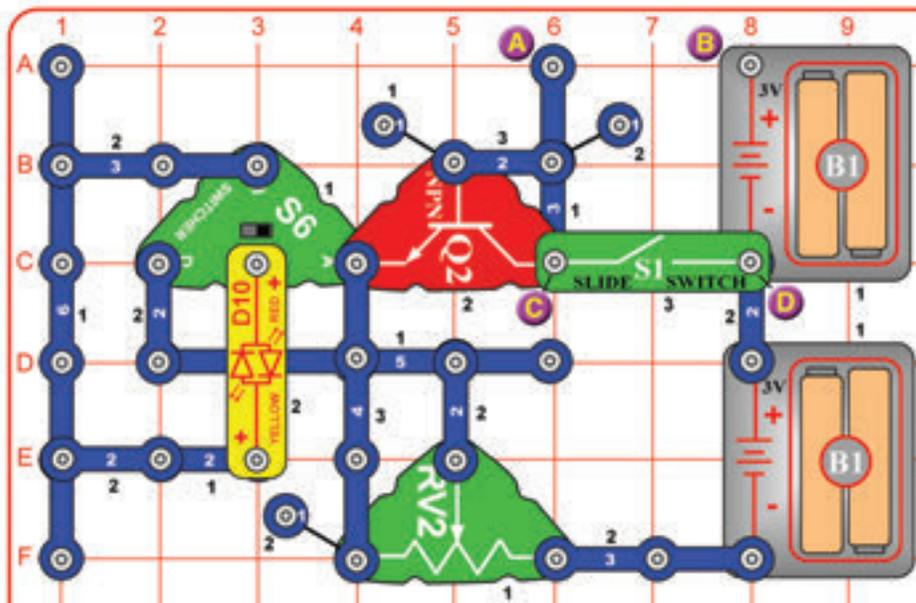
Turn on the slide switch (S1). Set the switcher (S6) to both the left & right positions at several settings on the adjustable resistor (RV2), and compare the brightness of the red/yellow bicolor LED (D10). See if you can notice a difference in the LED brightness between red and yellow, especially when the LED is very dim.
