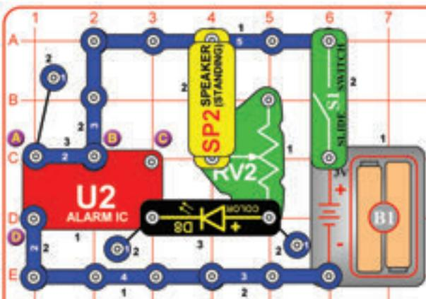
Build the circuit and turn on the slide switch (S1). Use the lever on the adjustable resistor (RV2) to change the sound volume and light brightness.
