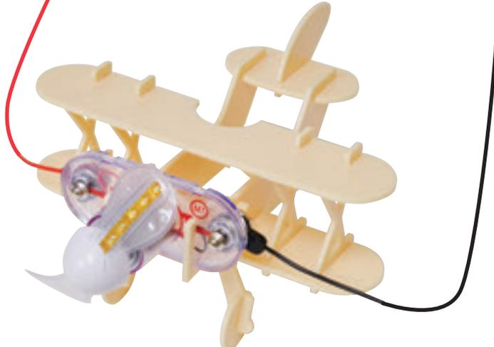
This circuit runs the air fountain (AF) at 3V instead of 6V. Now the air fountain doesn't operate at full power, but it uses less current from the batteries. The lower current here will rarely (or never) activate the fuse like it could in the preceding project, and if the fuse does activate it would only be after a much longer operating time.
