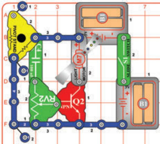
Set the adjustable resistor (RV2) to the top setting and keep it there. Turn on the slide switch (S1). The fan on the light motor (M7) spins briefly and stops. Now turn off the slide switch, wait a little while, and then turn it back on. The fan spins briefly again. Try this several times.
