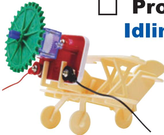
Use either of the two preceding circuit, but replace the light motor (M7) with the geared motor (GM). Place the 2.55" gear on the "+" shaft of the geared motor, and mount the geared motor on the plane as shown.
