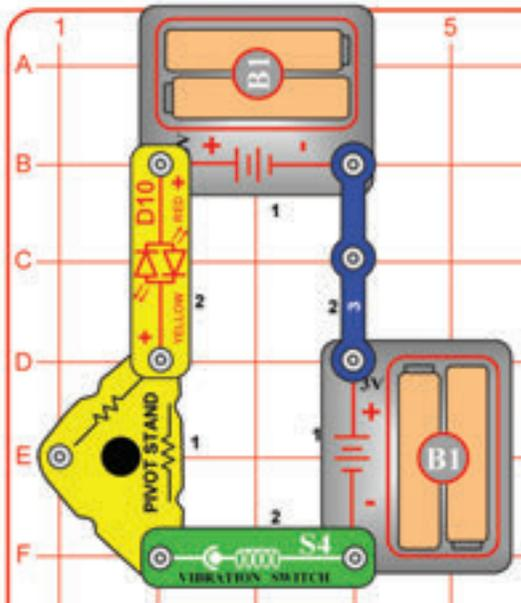
Build the circuit as shown. Tap on the vibration switch (S4) or bang on the table to make the red/yellow LED (D10) light.
