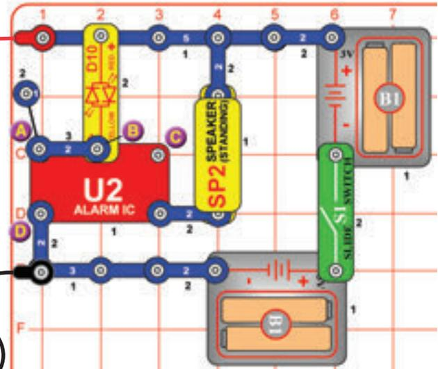
Assemble the airplane using the instructions on page 5, install the light motor (M7) into the front of it, build the circuit shown here, and connect the red & black jumper wires to the light motor (red to "+"). Spread out the jumper wires and be sure they will not interfere with the fan on the light motor.
