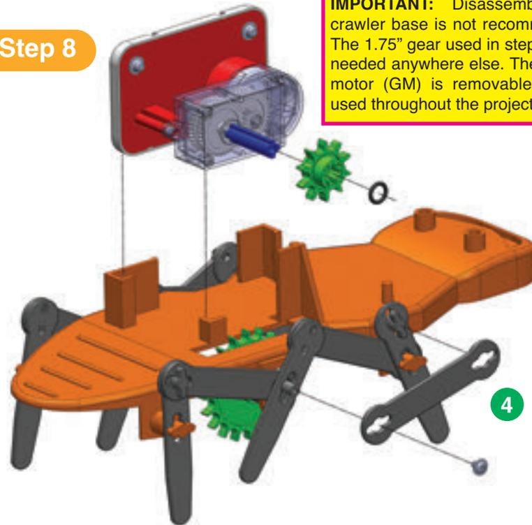
**IMPORTANT:** Disassembling the crawler base is not recommended. The 1.75" gear used in step 1 is not needed anywhere else. The geared motor (GM) is removable, and is used throughout the projects.
