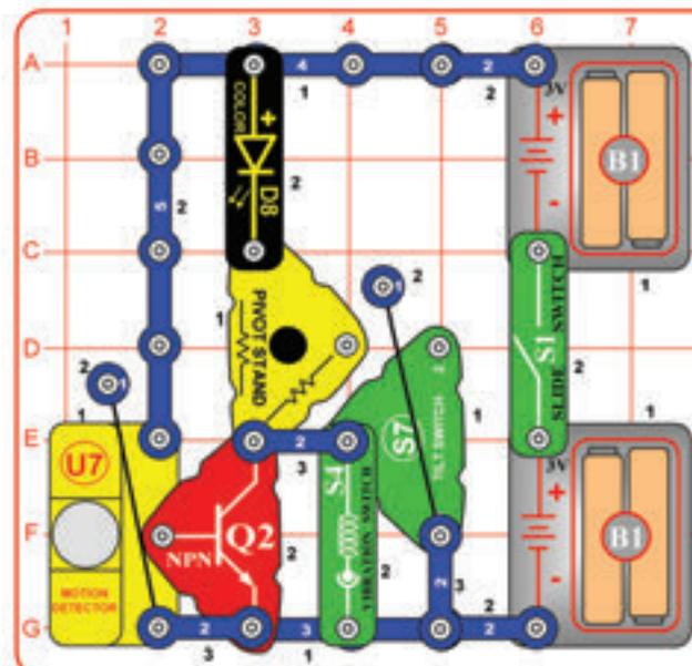
Build the circuit and turn on the slide switch (S1). The color LED (D8) lights for a few seconds on start-up, and then whenever the circuit detects motion, feels vibration, or is tilted in some directions.
