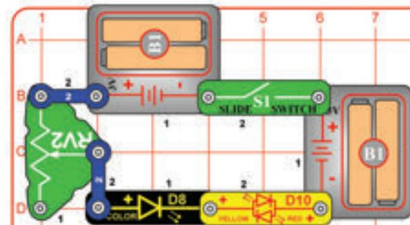
Turn on the slide switch (S1) and adjust the brightness of both LEDs (D8 & D10) using the lever on the adjustable resistor (RV2). You can flip D10 around to change its color from yellow to red.
