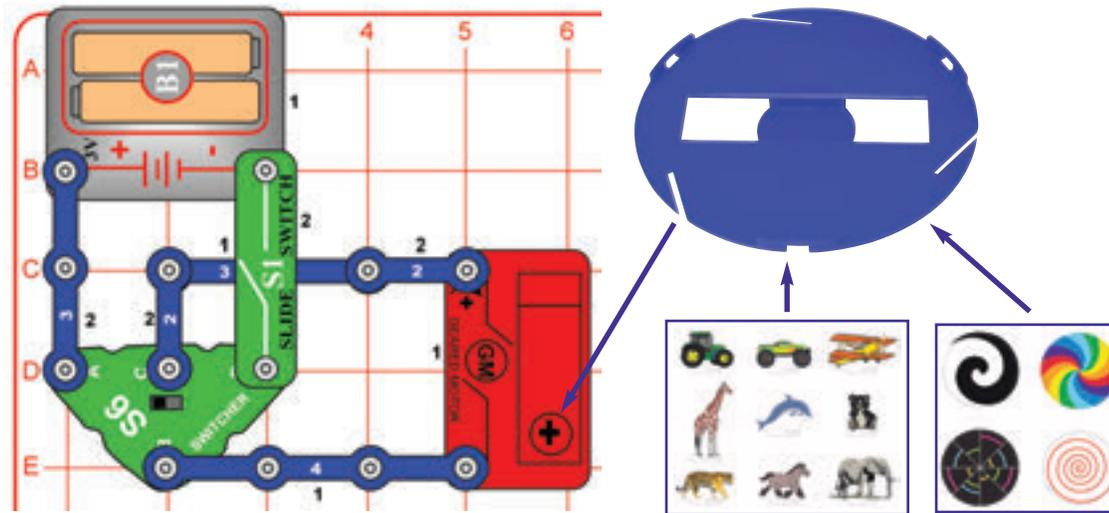
Either insert some of the cardboard figures into the 3 slots on the edge of the merry-go-round base, or install one of the colored discs into the base. Build this circuit and mount the merry-go-round base onto the shaft on the geared motor (GM).
