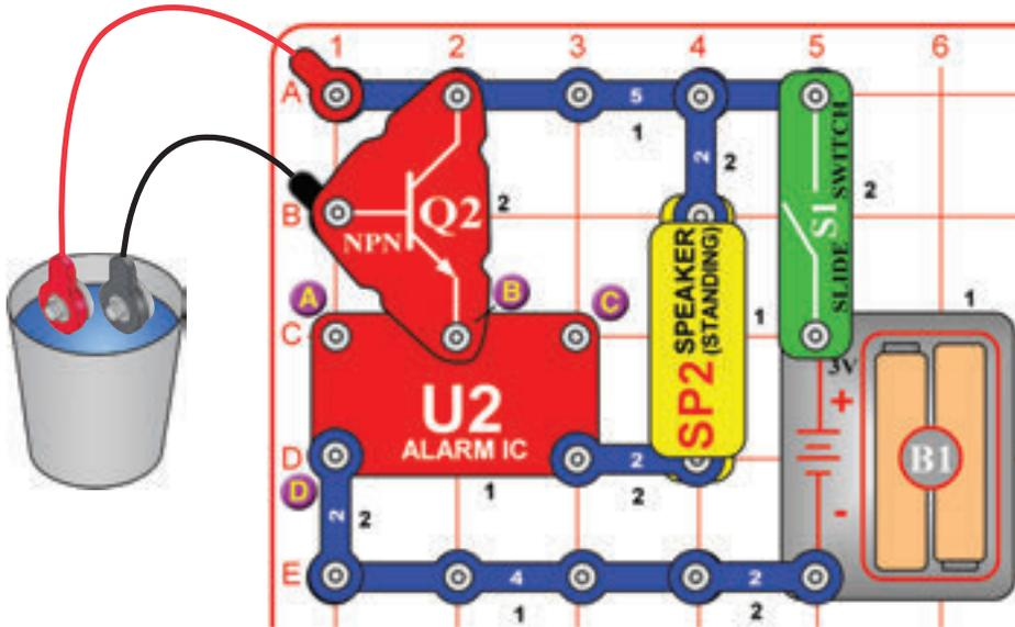
Build the circuit shown but initially leave the red & black jumper wires outside the cup. Turn on the slide switch (S1); nothing happens. Place the jumper wires into a cup of water and an alarm sounds!
