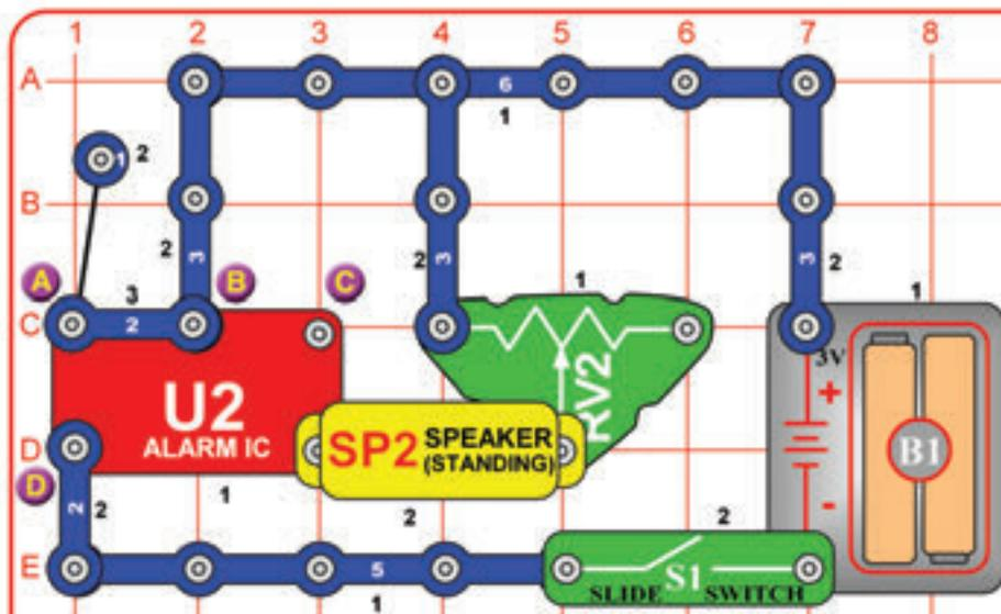
The preceding circuit may be too loud, so modify it to match this one, which uses the adjustable resistor (RV2) as a volume control. Turn on the slide switch (S1) and adjust the volume using RV2.
