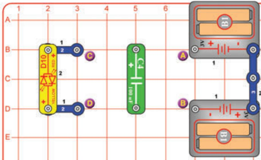
This circuit has two parts; build it as shown, but initially place the 100 $\mu$ F capacitor (C4) across points A & B. Then pick up C4 and place it across points C & D; the red/yellow bicolor LED (D10) flashes. Move C4 between points A/B & C/D several times.
