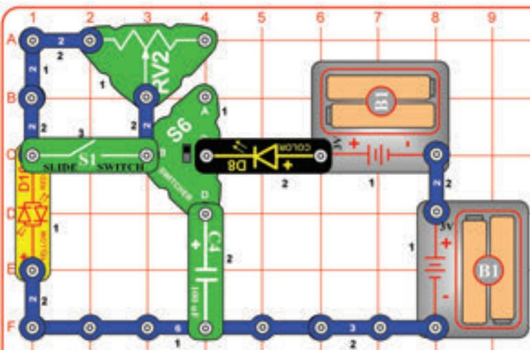
Modify the preceding circuit to match this one. Turn off the slide switch (S1); now the adjustable resistor (RV2) controls how quickly the 100µF capacitor (C4) discharges through the red/yellow LED (D10). Setting RV2 to the left makes D10 flash brightly but briefly; setting RV2 to the right makes the LED dimmer but it stays on longer.
