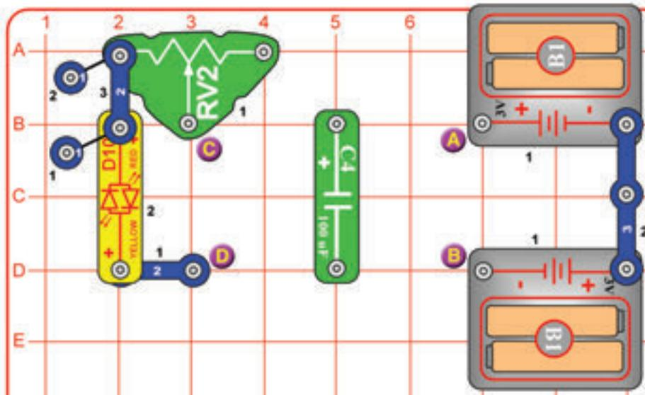
Modify the preceding circuit to match this one. It works the same way, except the adjustable resistor (RV2) slows down the capacitor discharge, making the LED dimmer but stay on longer. Try this at different RV2 settings.
