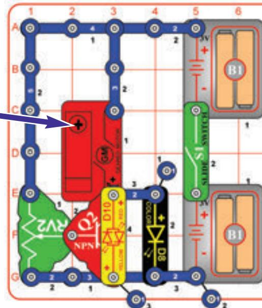
Modify the preceding circuit to make this one. Set the lever on the adjustable resistor (RV2) to the top. Turn on the slide switch (S1), and use the lever on the adjustable resistor to set the brightness of the LEDs (D8 & D10) and the speed of the merry-go-round base.
