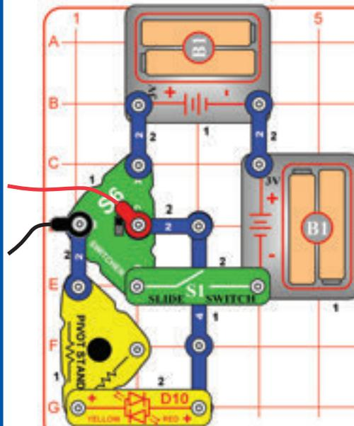
Modify the preceding circuit to use a second battery holder (B1), as shown. The crawler is much faster now.
