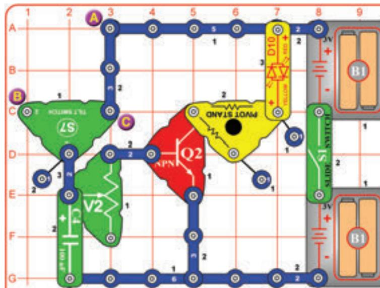
Modify the preceding circuit to be this one. Turn on the slide switch (S1). A light comes on if the circuit is moved, or tilted in some directions. The light stays on for a while after the tilt is removed. The lever on the adjustable resistor (RV2) controls how long the light stays on after tilt is removed.
