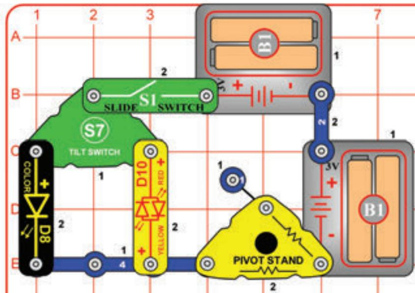
Build the circuit as shown and turn on the slide switch (S1). The color LED (D8) or red/yellow LED (D10) will light if the circuit is tilted or moved. Experiment to see which tilt angles activate which LED.
