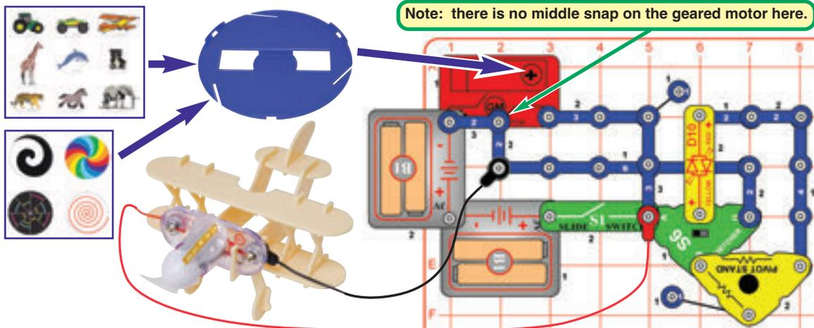
Modify the preceding circuit by removing the color LED (D8) and adding the second battery holder (B1) to the circuit as shown. Either insert some of the cardboard figures into the 3 slots on the edge of the merry-go-round base, or install one of the colored discs into the base. Mount the merry-go-round base onto the shaft on the geared motor (GM). Turn on the slide switch (S1).
