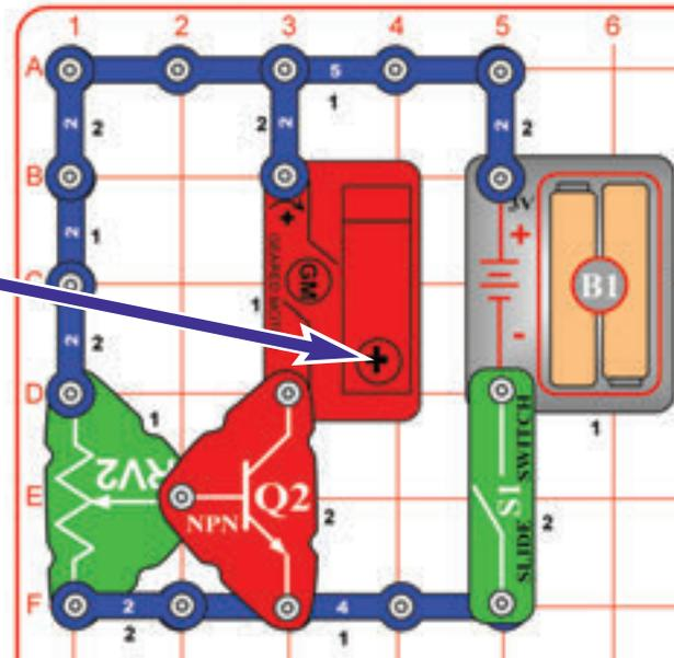
Insert some of the cardboard figures into the 3 slots on the edge of the merry-go-round base (the figures may need to be punched out of a cardboard sheet). Build this circuit and mount the merry-go-round base onto the shaft on the geared motor (GM).
