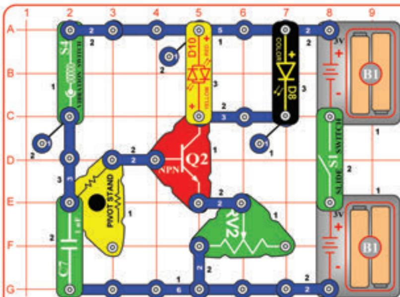
Build the circuit and turn on the slide switch (S1). Bang on the table or tap on the vibration switch (S4) and lights come on. The lights stay on for a while after the vibrations end. The lever on the adjustable resistor (RV2) controls the maximum light brightness and how long the lights stay on after vibrations end; the brighter the lights, the faster they shut off.
