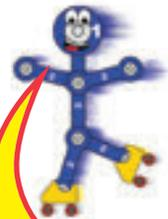
Rearrange the parts in the preceding circuit to make this one, which has them connected in a loop. Turn on the slide switch (S1). The LEDs (D8 & D10) light, but the geared motor (GM), air fountain (AF), and light motor (M7) do nothing. Snappy knows why.
