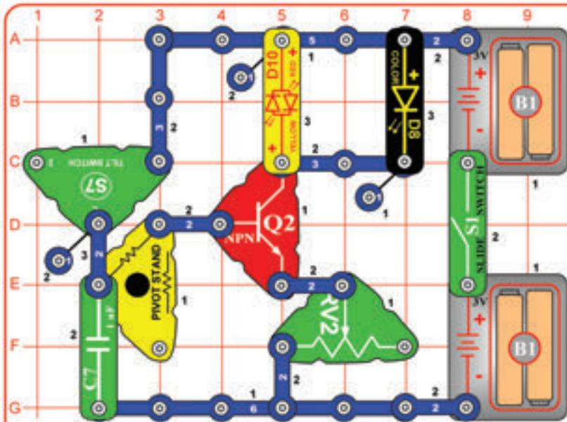
Build the circuit and turn on the slide switch (S1). Lights come on if the circuit is moved, or tilted in some directions. The lights stay on for a while after the tilt is removed. The lever on the adjustable resistor (RV2) controls the maximum light brightness and how long the lights stay on after tilt is removed; the brighter the lights, the faster they shut off.
