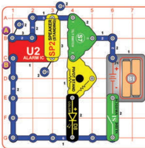
Build the circuit and turn on the slide switch (S1). A siren will sound or a light will shine if the circuit is tilted or moved. Experiment to see which tilt angles activate which effects.
