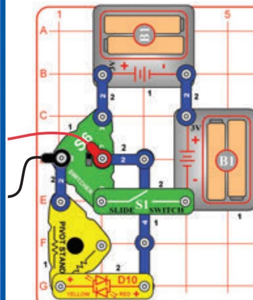
Modify the preceding circuit to use a second battery holder (B1), as shown. The car is much faster now, but more difficult to control.
