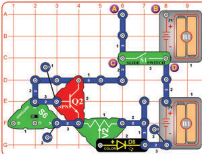
Set the switcher (S6) to the middle position and turn on the slide switch (S1). Set the lever on the adjustable resistor (RV2) all the way to the left. The color LED (D8) should be on, but may be mostly red. Slowly move the lever on RV2 to the right until the LED is completely off. Notice that the red color stays on the longest.
