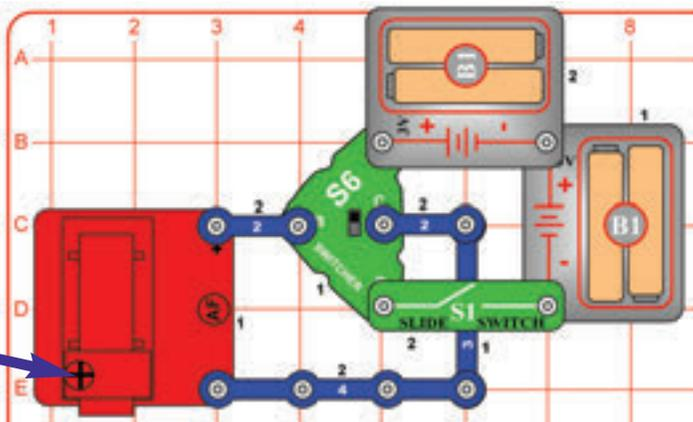
Build this circuit, turn on the slide switch (S1), set the switcher (S6) to either the top or bottom position, and place the ball in the air flow above the spout on the air fountain (AF). See how long the ball floats in the air for each S6 setting.
