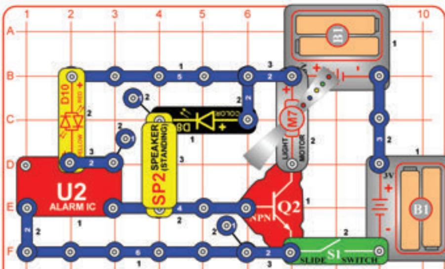
Build the circuit and turn on the slide switch (S1). The light motor (M7) spins in short bursts, synchronized with a machine gun-like sound.
