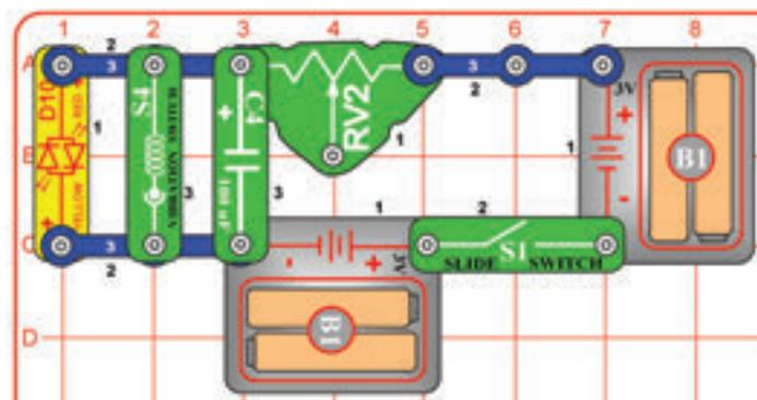
The vibration switch (S4) is connected so it bypasses the red/yellow bicolor LED (D10), so whenever vibrations turn on the switch, the LED turns off. However the vibrations occur so fast, turning off the LED so briefly that normally your eyes wouldn't even notice. The 1µF capacitor (C7) is used here to slow things down, so the LED does not immediately come back on after the vibration switch turned it off. If you remove C7, then you probably won't notice vibrations shutting off the LED (try it).
