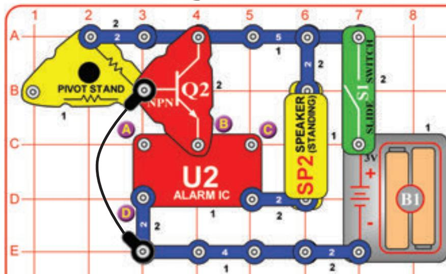
Build the circuit shown and turn on the slide switch (S1). Nothing happens. Break the black jumper wire connection and an alarm sounds. You could replace the black jumper wire with a longer wire and run it across a doorway to signal an alarm when someone enters.
