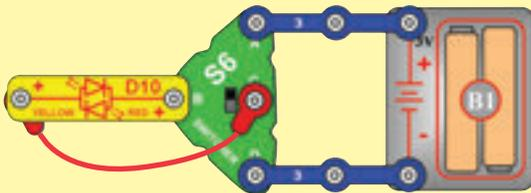
14. **1 $\mu$ F (C7) and 100 $\mu$ F (C4) capacitors:** Build project 139. Touch C4 or C7 across points A & B, then across points C & D; the LED (D10) should flash (brightly for C4 and dimly for C7) or the capacitor is broken.
