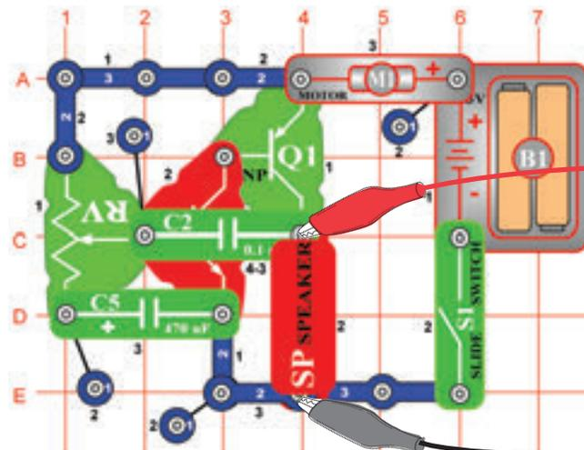
Build the circuit shown. If continuing from the previous experiment then close the Winscope program and run it again, to reset the settings. Click on the **On-Line** button to activate, and turn on the switch (snap part S1). Set Winscope to the settings shown below, and move the lever on the adjustable resistance (snap part RV) around to change **the waveform** and the sound. A sample waveform is shown here, but the pattern and shape of the pulses depends on the adjustable resistance setting.
