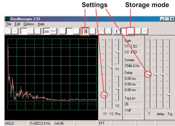
You can also turn on **Storage mode** to see the peaks recorded as you turn the motor, a sample of this is at right.
