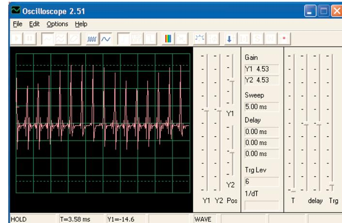
Winscope makes measurements using a 44kHz sampling rate, which is fast enough to measure the frequency of this signal (varying from 1-5kHz). However these pulses have much of their energy spread among higher frequencies that approach the sampling rate (see the sample spectrum plots at right), where the amplitude measurement becomes increasingly inaccurate.
