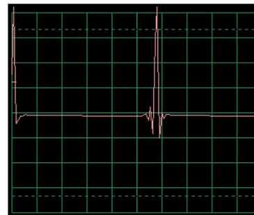
The waveform above is weak and erratic, so replace the 0.02μF capacitor (snap part C1) with the 0.1μF capacitor. A sample of the new waveform is at left, with the same settings. It is lower in frequency but higher in amplitude.
