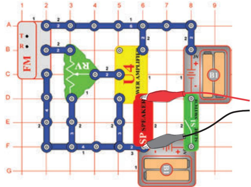
Turn on the switch (S1) and press the R button. Now press the T button and FM module scans for a radio station. When a station is found, it locks on to it and you hear it on the speaker. Press the T button again for the next radio station.
