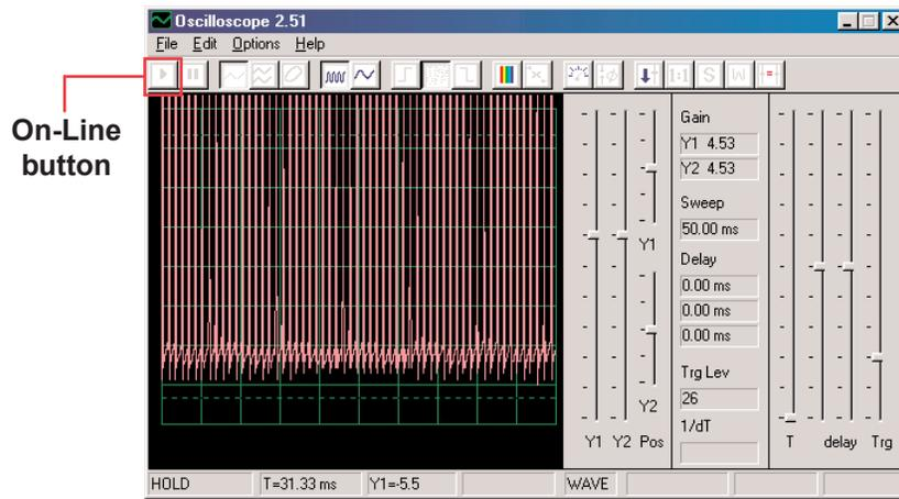
The waveform peak is off the top of the screen because the scope gain (amplification) is set too high. You may adjust this gain by moving the **Y1 gain control** around (try it).
