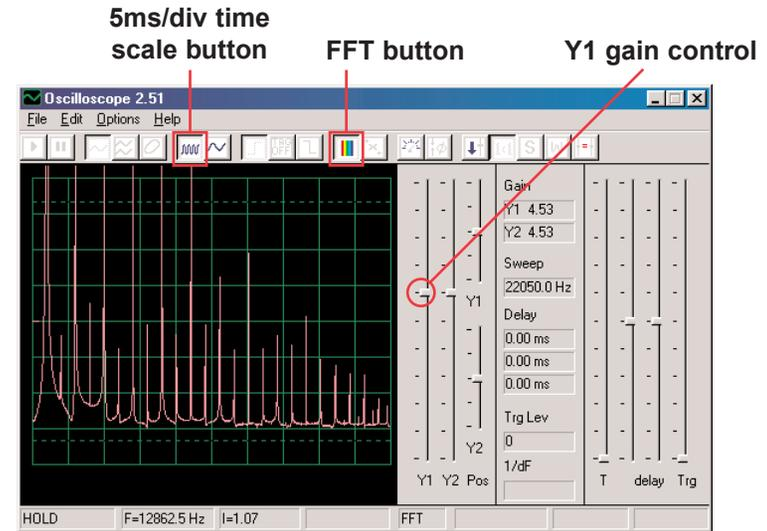
Note that the sound is music and the oscilloscope waveform has a “square” shape, as a result the frequency spectrum has a lot peaks with equal spacing.
