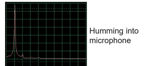
The above frequency spectrum pictures correspond directly to the waveform pictures on the preceding page. Notice that the spectrums for the hum and whistle have only a single big peak. Smooth, well-rounded, and repetitive waveforms (in oscilloscope
