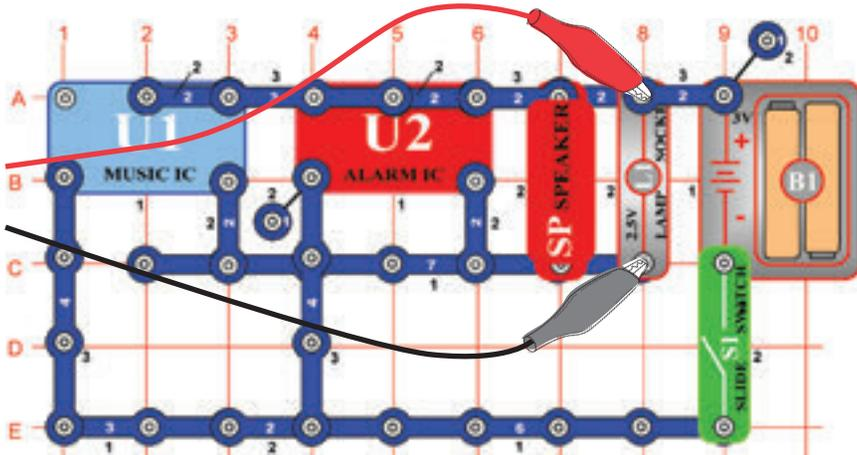
Build the circuit and try the **settings** shown. Turn it on and view the waveforms.
