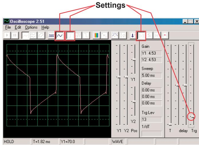
Note that in the above display the Y1 Gain is set high to show the low energy levels of the signal, even though the stronger peaks of the lower frequency components are off the top of the display. This can be deceiving. Now change the **Y1 Gain** so that the highest peak can be seen, this is shown on the right. Now you see how the main signal frequency dominates the others.
