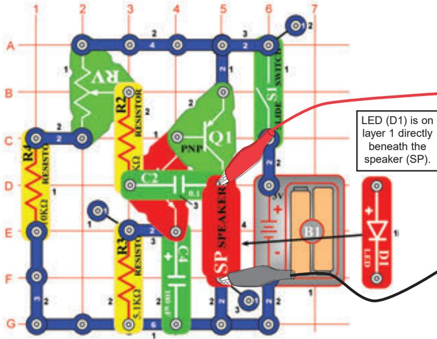
Build the circuit shown. If continuing from the previous experiment then close the Winscope program and run it again, to reset the settings. Click on the On-Line button to activate, and turn on the switch (snap part S1). Set Winscope to the **settings** shown on the upper right, and move the lever on the adjustable resistance (snap part RV) around to change the waveform and the sound. At some positions there may be no sound. A sample waveform is shown on the upper right.
