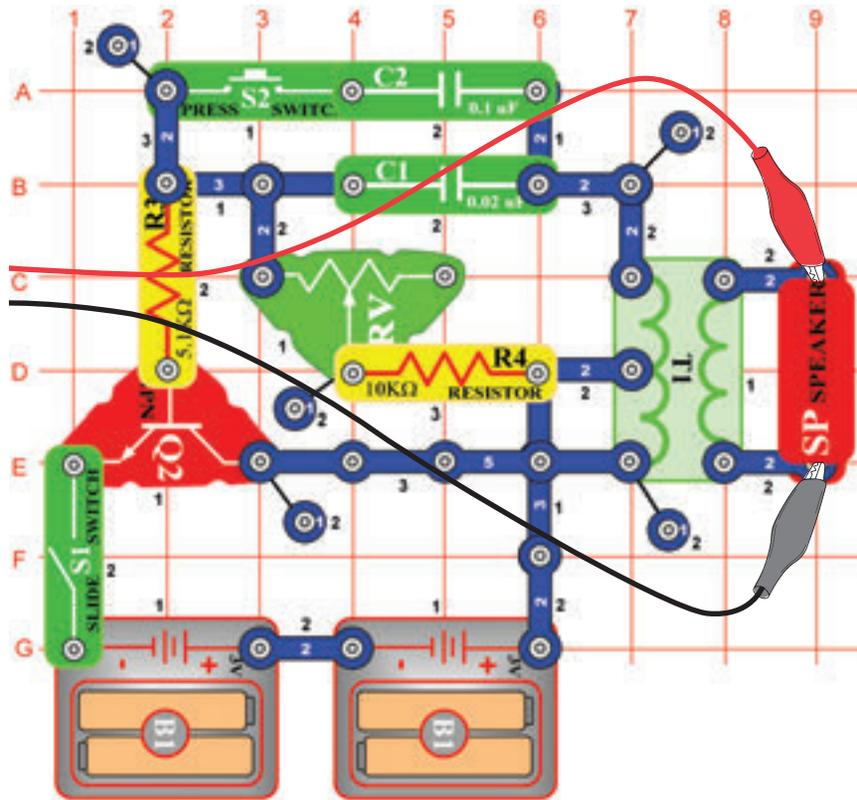
Build the circuit and try the settings shown. Flip on the slide switch and press the press switch a few times while moving the variable resistor control around. View the waveform and frequency spectrum.
