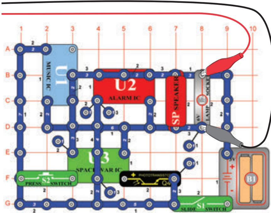
The Symphony of Sounds project combines waveforms from the Music, Alarm, and Space War integrated circuits. Build the circuit shown. If continuing from the previous experiment then close the Winscope program and run it again, to reset the settings. Click on the On-Line button to activate, and turn on the switch (snap part S1). Press the press switch (S2) and wave your hand over the phototransistor (Q4).
