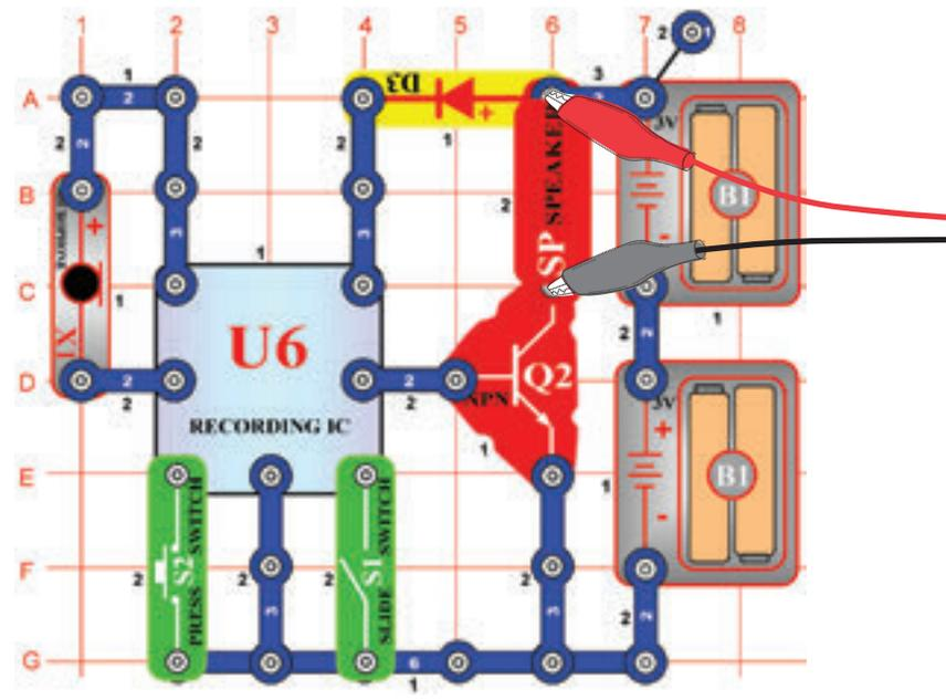
Build the circuit shown. Turn on the switch (S1), you hear a beep signaling that you may begin recording. Talk into the microphone (X1) up to 8 seconds, and then turn off the switch (S1) (it also beeps after the 8 seconds expires).
