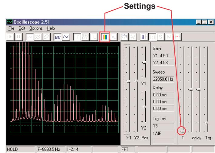
The spectrum at left is for just after pressing the press switch. The spectrum below uses the same settings and shows the spectrum just before the sound stops. The frequencies and amplitude slowly get lower as the sound fades away.
