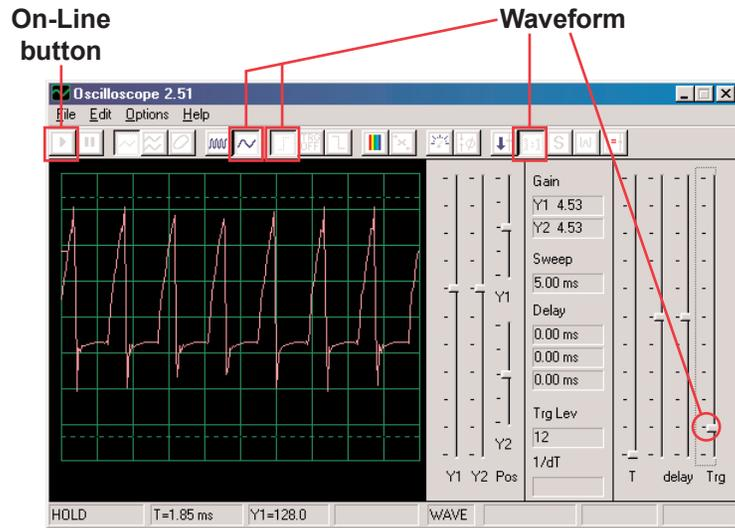
Winscope has a mode that can display multiple scans at the same time, called **Storage mode**. Set the adjustable resistance lever to a low-middle position, place Winscope in this mode, and watch the results.
