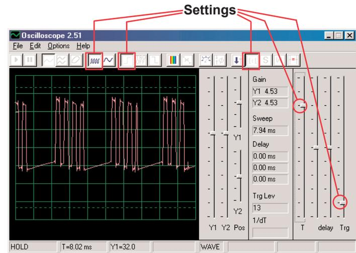
The oscilloscope display alternates between 2 waveforms, the one shown here and the one on the next page. This one shows some pulses followed by a flat signal, then more pulses, then flat, then pulses, then flat . . .
