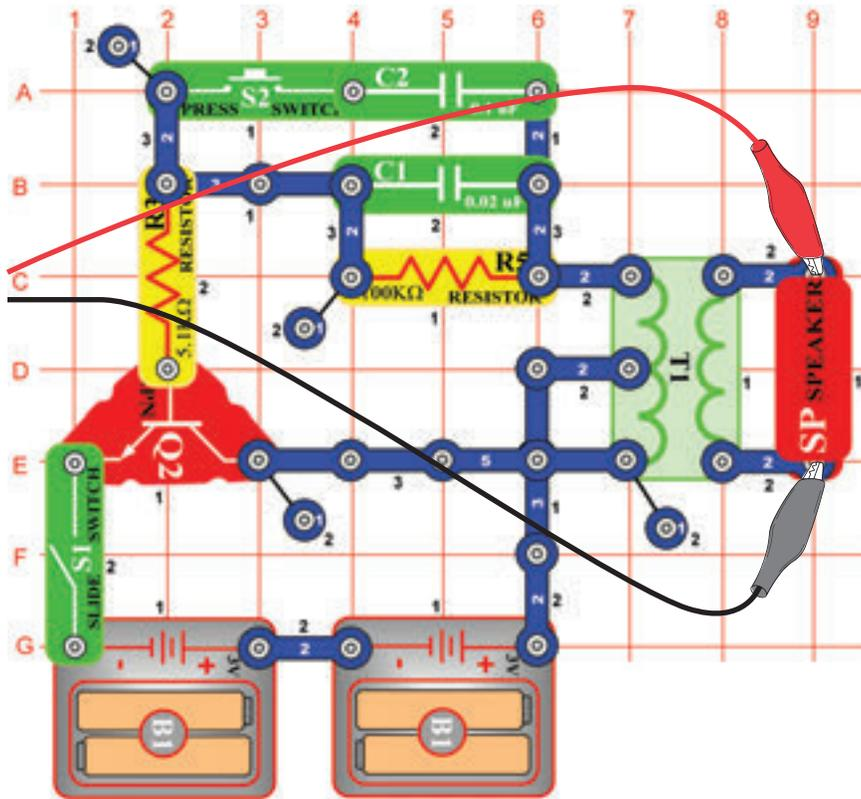
Build the circuit and try the **settings** shown. Press the press switch to lower the frequency of the signal by increasing the capacitance in the oscillator. You can replace the  $0.1\mu\text{F}$  capacitor C2 with the  $10\mu\text{F}$  capacitor C3 to further lower the frequency of the tone. You may try other settings to zoom in or look at the frequency spectrum.
