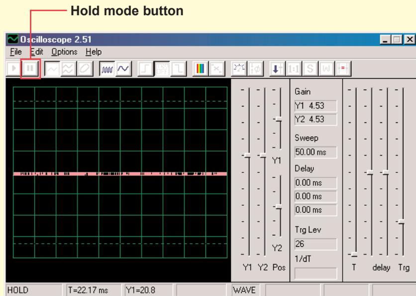
**WARNING:** Do not “save setup” in Winscope. Many of the buttons on Winscope control features that this manual will not be using. If you accidentally place the Winscope software into an unknown mode, you may always close and re-start Winscope. Doing so will reset all settings to those described in this booklet unless you have done a “save setup”.
