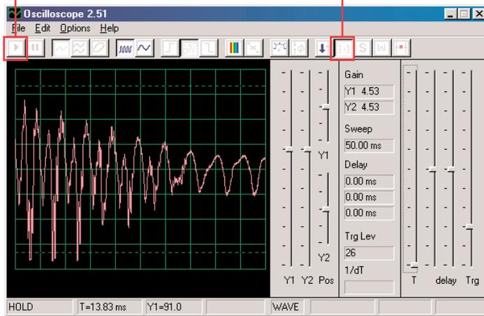
You should see a waveform similar to that shown here, but it will be constantly changing as the music or talking you hear is changing. Try tuning the adjustable capacitor (snap part CV) to different radio stations and compare the waveforms.
