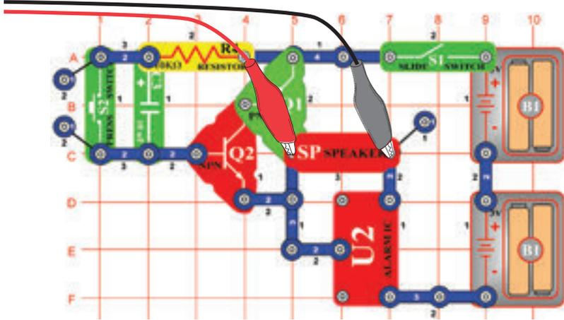
Build the circuit shown. If continuing from the previous experiment then close the Winscope program and run it again, to reset the settings. Set Winscope to the **settings** shown on the right. Click on the On-Line button to activate, turn on the switch, and press the press switch (snap part S2). You hear a siren that slowly fades away.
