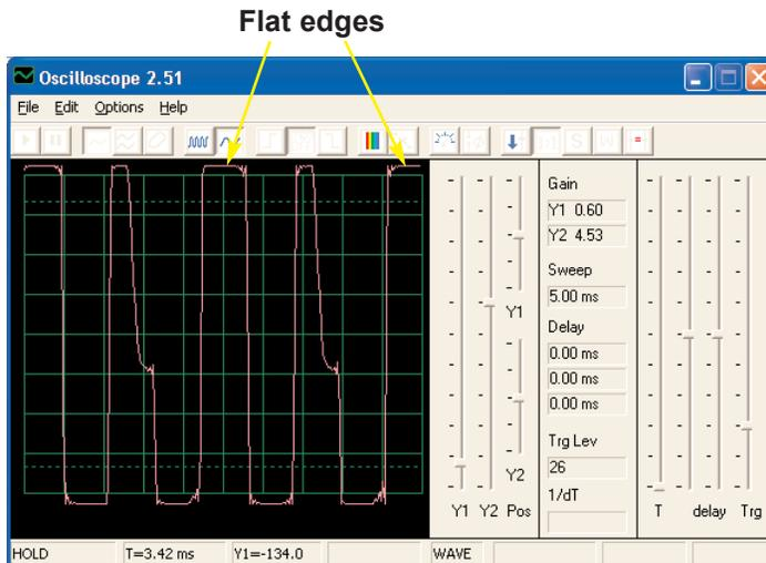
Set the variable resistor to the bottom position and turn on the switch, you will see a waveform like that shown below. Set the variable resistor to the top, and the waveform looks like that shown on the bottom left, due to lower resistance in the circuit. A sample frequency spectrum is also shown on the bottom right.
