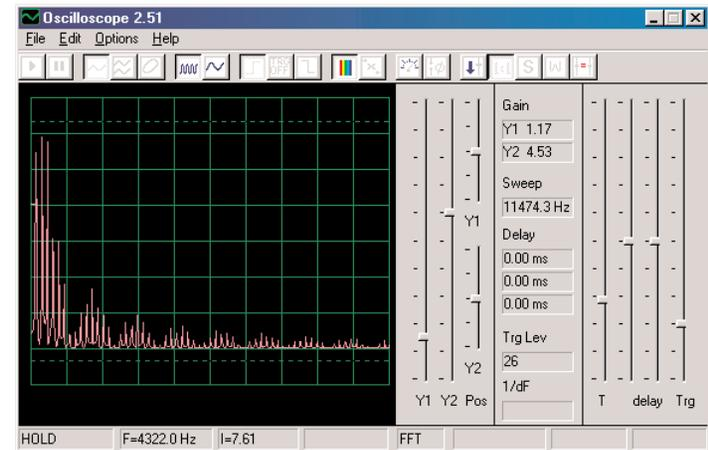
Now adjust the **horizontal scale** so the peaks line up with the gridlines as they did before.
