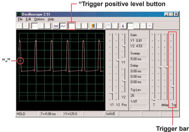
The small slash **“-”** represents the trigger voltage, when the signal reaches this voltage level it activates the display. This makes it easy to observe a stream of pulses like you have now, and also to record a single (non-repeating) pulse.
