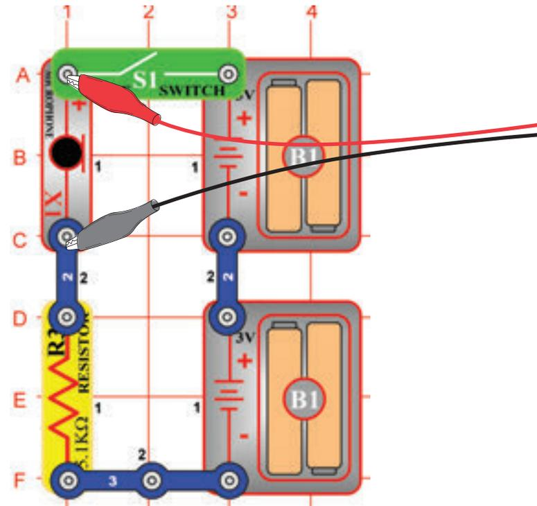
If continuing from the previous experiment then close the Winscope program and run it again, to reset the settings. Click on the **On-Line** button to activate Winscope, and turn on the switch (snap part S1).
