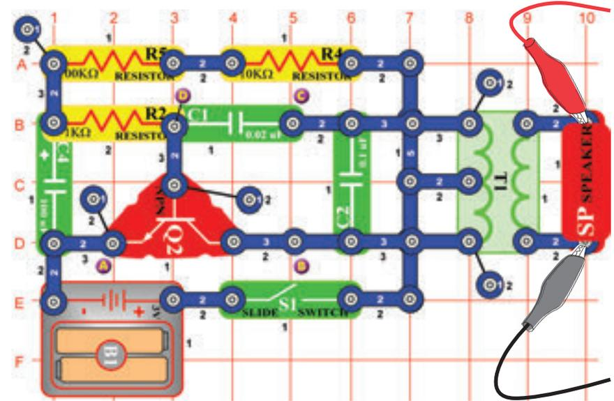
Build the circuit and try the **settings** shown. The oscillator activates about once-a-second, sounding like a bird chirping. You may look at the frequency spectrum if you like.
