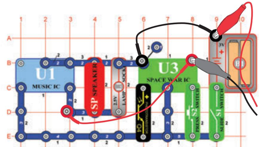
Build the circuit and try the settings shown. Turn it on, press the press switch (S2) several times, and wave your hand over the phototransistor (Q4) to view all the sound combinations. Compare the waveform and spectrum to the alarm IC combo circuit.
