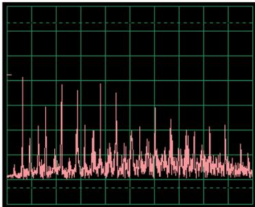
Now put the 0.02µF capacitor back in place of the 0.1µF capacitor to compare its spectrum. A sample is on the left, with the same Winscope settings as above. As with the oscilloscope mode, its spectrum is weaker and more erratic.
