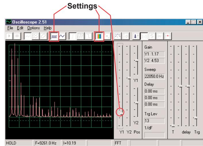
You can change some of the Winscope settings around to view the waveform and spectrum in different ways if desired. You can also place the 0.02 $\mu$ F capacitor on top of the whistle chip to lower the frequency.
