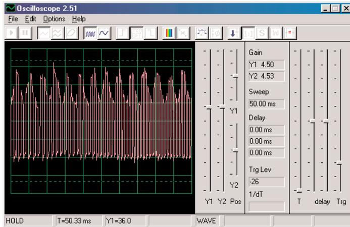
The waveform shown here is from humming into the microphone, notice how the tops of the pulses show a regular pattern of dips now.
