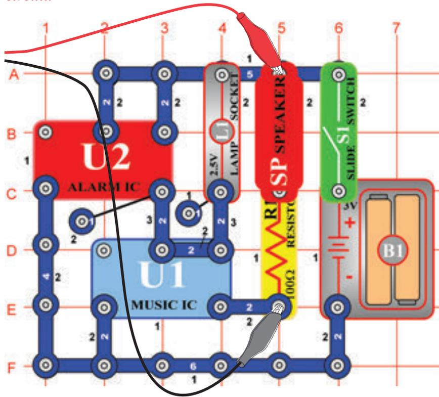
Build the circuit shown. If continuing from the previous experiment then close the Winscope program and run it again, to reset the settings. Click on the On-Line button to activate, and turn on the switch (snap part S1). Try the **settings** shown here.
