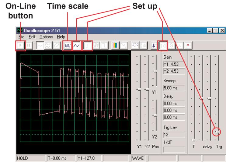
Press the press switch (snap part S2) several times to step through the eight different sounds from the space war integrated circuit. Hold it down for a few seconds each time so you can see the waveform representing the sound you hear.
