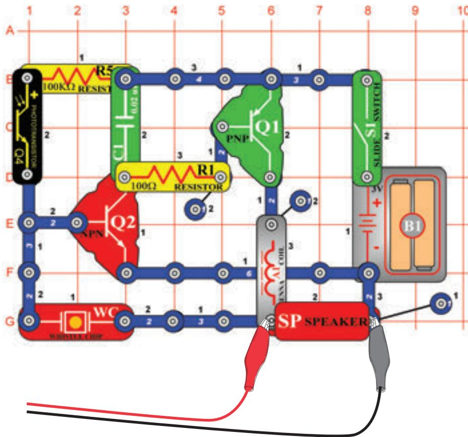
Build the circuit shown. If continuing from the previous experiment then close the Winscope program and run it again, to reset the settings. Set Winscope to the **settings** shown below and click on the On-Line button to activate. A sample waveform is shown here.
