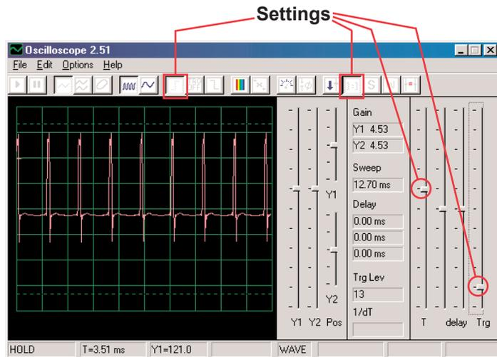
The waveform at left shows the signal just after pressing the press switch, the waveform below uses the same settings and shows the waveform just before the sound stops. You see the pulses slowly spread out as the tone of the sound changes.
