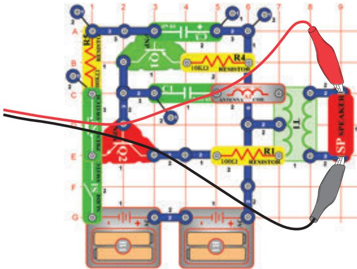
Build the circuit and try the **settings** shown. Flip on the slide switch and press the press switch for a few seconds and release. View the waveform as a siren starts up and then slowly fades away.
