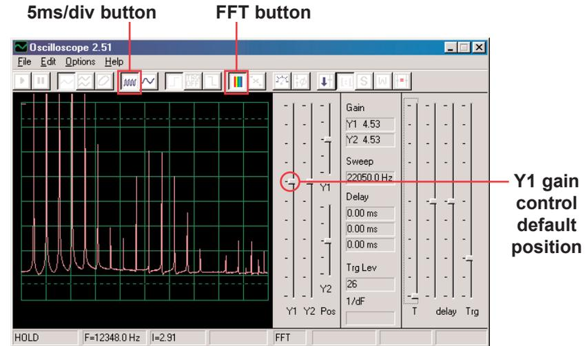
You are seeing the frequency spectrum of your signal, up to 22kHz. Notice that most of the energy is at the low frequencies (below 7kHz), and there is very little as you go higher.
