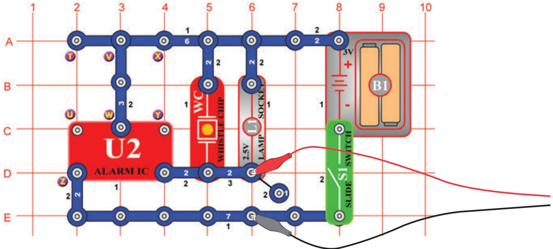
Build the circuit and connect the Winscope PC-interface cable as shown, the cable should still be connected to the microphone input on your computer.
