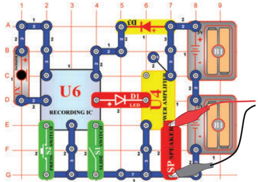
Build the circuit shown. Turn on the switch (S1), you hear a beep signaling that you may begin recording. Talk into the microphone (X1) up to 8 seconds, and then turn off the switch (S1) (it also beeps after the 8 seconds expires).
