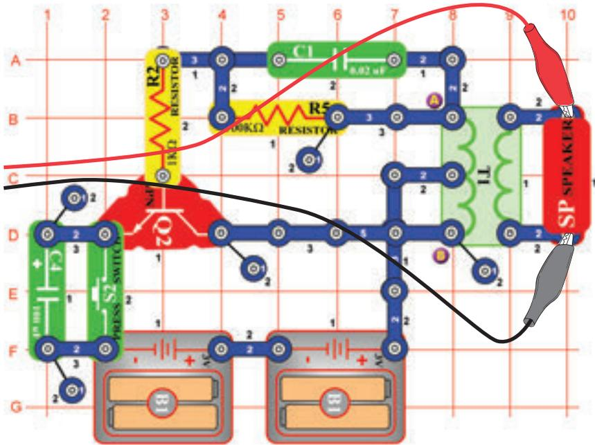
Build the circuit and press the press switch a few times, you hear cute sounds like a bumble bee. Use Winscope to see how the waveform fades away after you release the switch, and try **storage mode** as shown here.
