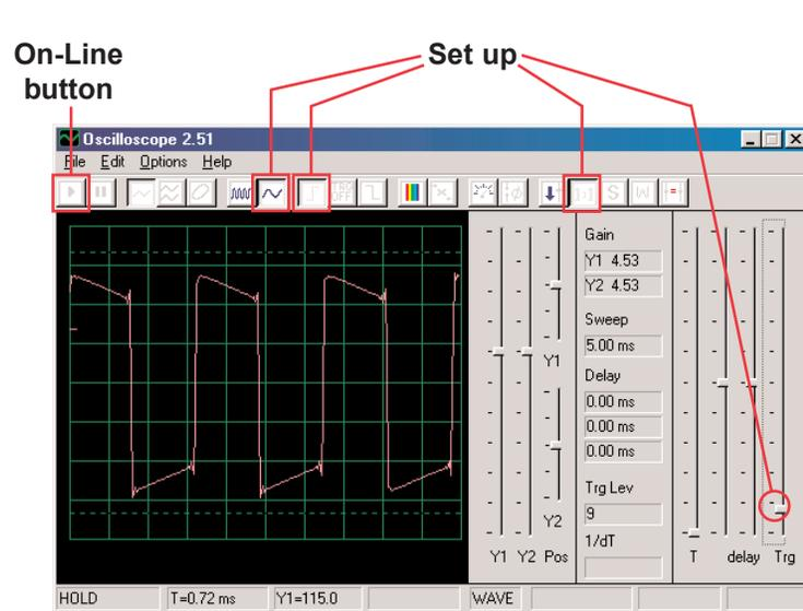
You should see a waveform similar to that shown here, but it will be constantly changing. This is because the siren sound you hear is not a continuous tone but instead is constantly changing. Note the differences in the waveshape for this circuit compared to the circuit in Project PC1.
