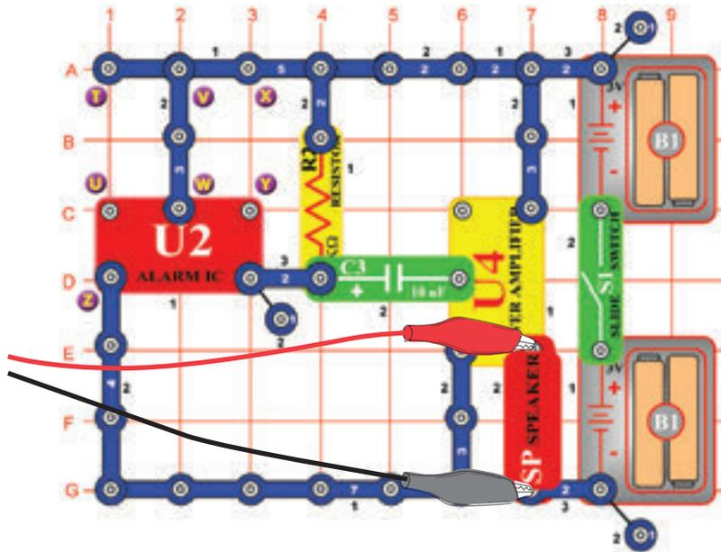
Build the circuit shown and set Winscope to the **settings** shown below. The siren sound is very loud. In most cases the waveform will have **flat edges** on the top and bottom, indicating the voltage is too high for the microphone input stage on your computer and is being distorted. You may sometimes correct for this if you like by reducing the volume control of your microphone input (see p. 4), but it is recommended that you return the volume to the normal level before doing other projects.
