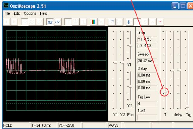
Build the circuit and try the **settings** shown. Start with the variable resistor set to the left but then adjust to change the tone. The signal dies out after you release the switch.
