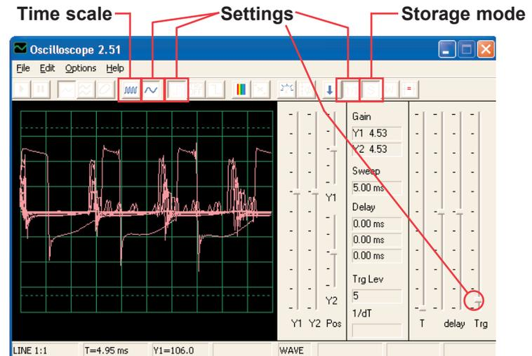
You may replace the  $0.02\mu\text{F}$  capacitor C1 with  $0.1\mu\text{F}$  capacitor C2 or  $10\mu\text{F}$  capacitor C3 to change the sound, but you may want to change the **time scale**.
