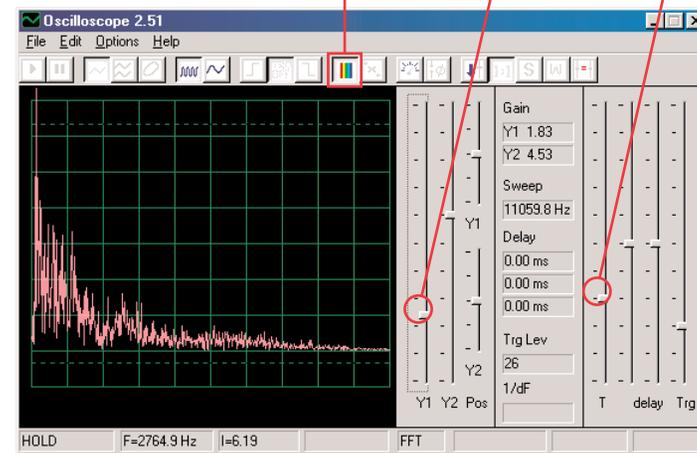
You should see a spectrum similar to that shown here, but it will be constantly changing as the music or talking you hear is changing. Try tuning the adjustable capacitor (snap part CV) to different radio stations and compare the waveforms.
