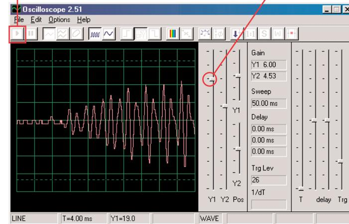
Notice that you need to set the gain control higher here than in the preceding project using the microphone, since speakers were not designed to be used in the same way.
