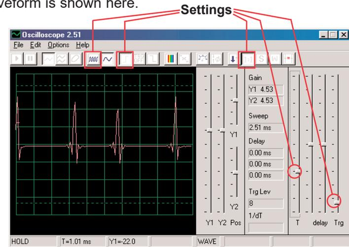
The actual waveform will vary depending on how much light is shining on the phototransistor (Q4). If you cover the phototransistor then the circuit shuts off.
