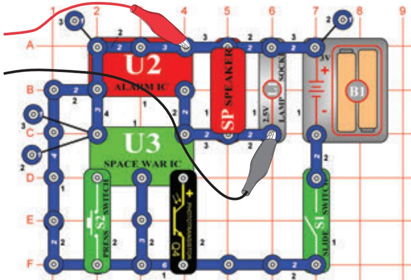
Build the circuit and try the settings shown. Turn it on, press the press switch (S2) several times, and wave your hand over the phototransistor (Q4) to view all the sound combinations. You may also use FFT mode to view the frequency spectrum.
