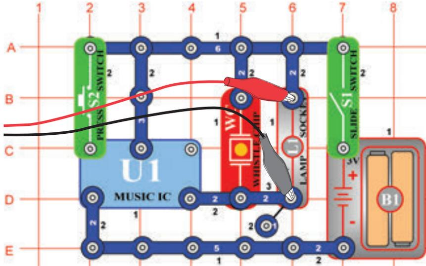
Build the circuit shown. If continuing from the previous experiment then close the Winscope program and run it again, to reset the settings. Click on the On-Line button to activate, and turn on the switch (snap part S1). Try the **settings** shown here. When the music stops, press the press switch (part S2) and it will resume.
