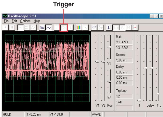
You can use Storage mode on any of the other circuit waveforms if desired.
