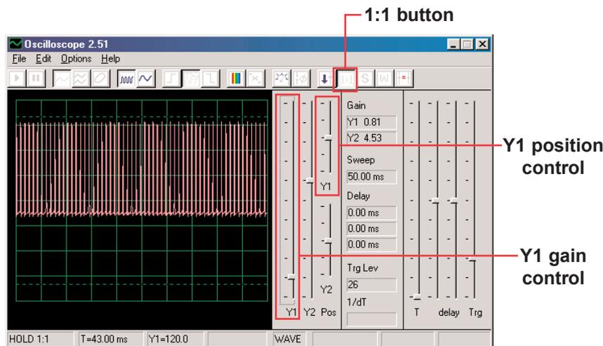
Note that your picture may not exactly match this picture due to variances in the microphone input gain between computers, which is beyond software control. You may want to adjust the volume control of your microphone input to compensate, see note A on page 4 for more details. You may also disable 1:1 mode by clicking on its button again and then adjust the gain using the Y1 control.
