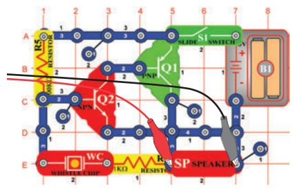
Build the circuit shown. If continuing from the previous experiment then close the Winscope program and run it again, to reset the settings. Click on the On-Line button to activate, and turn on the switch. Set Winscope to the **settings** shown below. A sample waveform is shown here.
