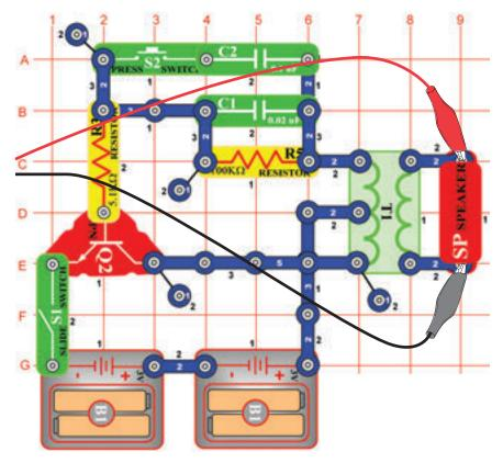
Build the circuit and try the **settings** shown. Press the press switch to lower the frequency of the signal by increasing the capacitance in the oscillator. You can replace the  $0.1\mu$ F capacitor C2 with the  $10\mu$ F capacitor C3 to further lower the frequency of the tone. You may try other settings to zoom in or look at the frequency spectrum.
