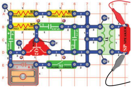
Build the circuit and try the **settings** shown. The oscillator activates about once-a-second, sounding like a bird chirping. You may look at the frequency spectrum if you like.
