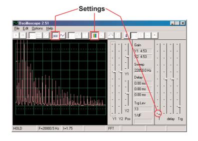
Note that in the above display the Y1 Gain is set high to show the low energy levels of the higher frequency components of the signal, even though the stronger peaks of the lower frequency components are off the top of the display. This can be deceiving. Now change the Y1 Gain so that the highest peak can be see, this is shown on the right. Now you see how the main signal frequency dominates the others.
