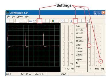
You may look at a pulse close-up by changing the **time scale** and slightly adjusting the **delay**, as shown.
