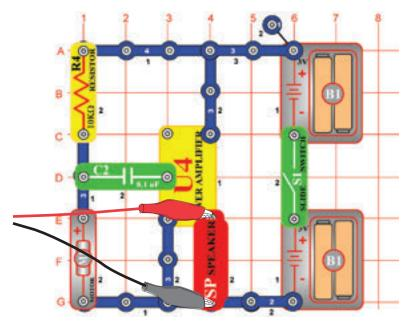
Build the circuit shown. If continuing from the previous experiment then close the Winscope program and run it again, to reset the settings. Click on the On-Line button to activate, and turn on the switch. Set Winscope to the **settings** shown on the upper right. Turn the motor (snap part M1) slowly with your fingers and watch the waveforms generated. They are very erratic and unpredictable. A sample is shown on the upper right.
