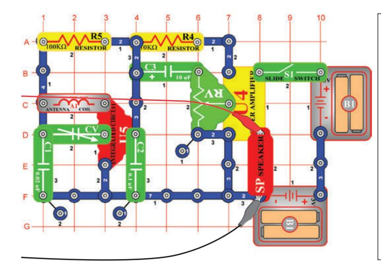
Build the circuit shown and connect PC-interface cable to the microphone input on your computer. Turn on the switch (snap part S1), tune the adjustable capacitor (snap part CV) to a local radio station that gives good reception, and set the adjustable resistance (snap part RV) to a comfortable loudness level. The integrated circuit (snap part U5) detects and amplifies the AM radio waves all around you. The power amplifier (snap part U4) drives the speaker to complete the circuit.
