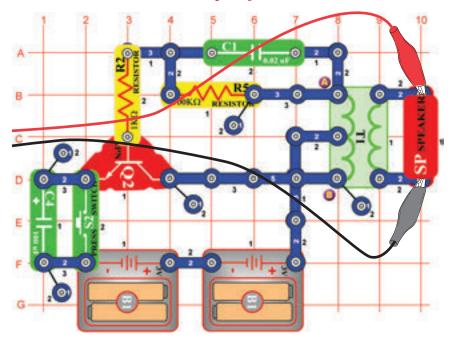
Build the circuit and press the press switch a few times, you hear cute sounds like a bumble bee. Use Winscope to see how the waveform fades away after you release the switch, and try **storage mode** as shown here.
