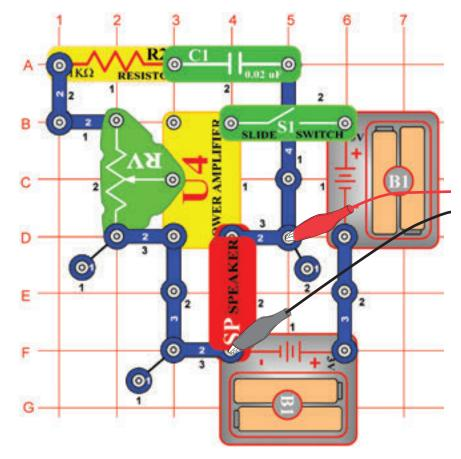
Build the circuit shown. If continuing from the previous experiment then close the Winscope program and run it again, to reset the settings. Click on the On-Line button to activate, and turn on the switch (snap part S1). Set Winscope to the **settings** shown below, and move the lever on the adjustable resistance (snap part RV) around to change the waveform and the sound. At some positions there may be no sound. A sample waveform is shown here.
