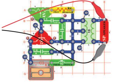
Build the circuit and try the **settings** shown. Start with the variable resistor set to the left but then adjust to change the tone. The signal dies out after you release the switch.
