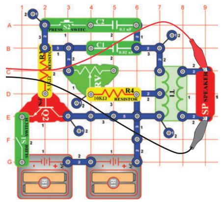
Build the circuit and try the settings shown. Flip on the slide switch and press the press switch a few times while moving the variable resistor control around. View the waveform and frequency spectrum. Sample frequency spectrum:
