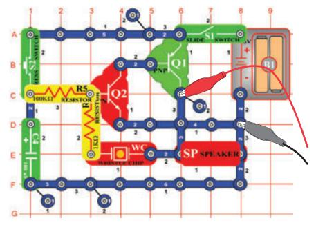
Build the circuit shown. If continuing from the previous experiment then close the Winscope program and run it again, to reset the settings. Click on the On-Line button to activate, turn on the switch (snap part S1), and press the press switch (part S2). Try the **settings** shown here.
