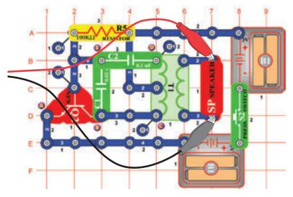
Build the circuit and try the **settings** shown here. This circuit produces a series of pulses (shown below), representing when the transistor is activated.
