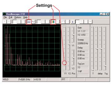
You can change some of the Winscope settings around to view the waveform and spectrum in different ways if desired. You can also place the  $0.02\mu$ F capacitor on top of the whistle chip to lower the frequency.
