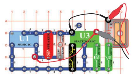
Build the circuit and try the **settings** shown. Turn it on, press the press switch (S2) several times, and wave your hand over the phototransistor (Q4) to view all the sound combinations. Compare the waveform and spectrum to the alarm IC combo circuit.
