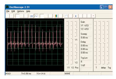
Winscope makes measurements using a 44kHz sampling rate, which is fast enough to measure the frequency of this signal (varying from 1-5kHz). However these pulses have much of their energy spread among higher frequencies that approach the sampling rate (see the sample spectrum plots at right), where the amplitude measurement becomes increasingly inaccurate.
