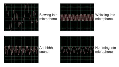
Click on the **FFT button** to look at the frequency spectrum for these signals. Try the **amplitude and time scales** shown here to start, but your best settings will depend on what sounds you make, how loud you speak, and how close you are to the microphone.
