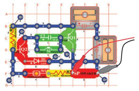
Build the circuit shown. If continuing from the previous experiment then close the Winscope program and run it again, to reset the settings. Click on the On-Line button to activate, and hold down the press switch (snap part S2). Set Winscope to the **settings** shown on the upper right. A sample waveform is shown on the upper right.
